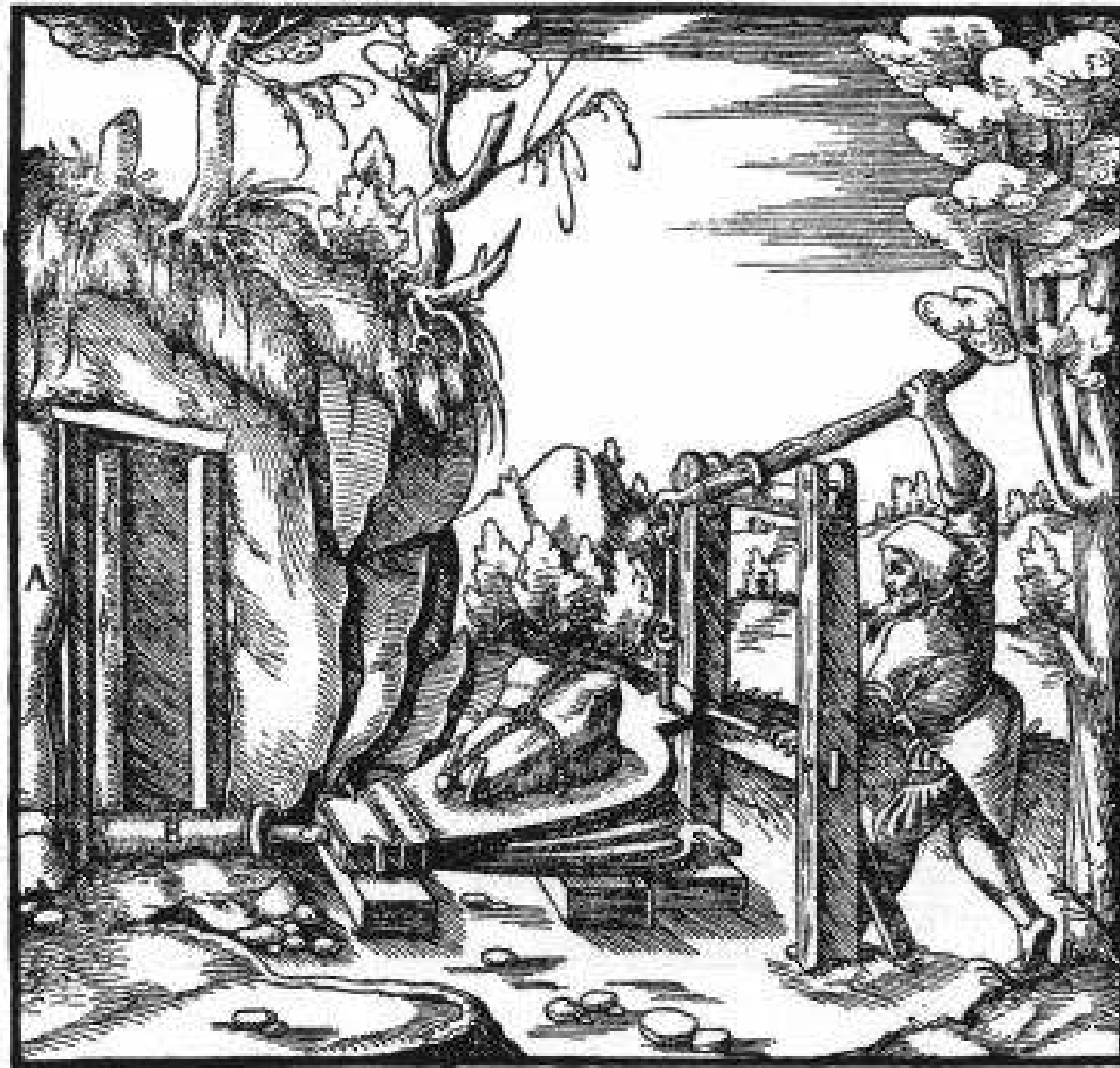
A—TUNNEL. B—PIPE. C—NOZZLE OF DOUBLE BELLOWS.
